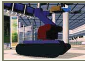
Operators can practise tricky operations like opening car doors and trunks, climbing stairs, and avoiding clumsy movements that might trigger an explosive device.
