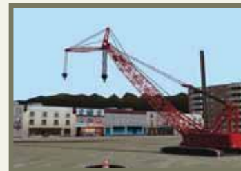
Vortex crawler crane simulator prepares students for dual-line operation with jib, plus clamshell, dragline, and even pile-driving operation.
