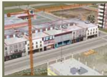
Vortex tower crane simulator allows operators to prepare for day-to-day tasks such as fly-forming, steel erection and concrete-bucket pouring.
