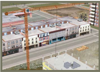
Vortex tower crane simulator allows operators to prepare for day-to-day tasks such as fly-forming, steel erection and concrete bucket pouring.
