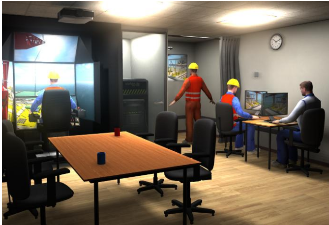
Vortex Crane Simulator installation for PNI Training Centre, showing team-based learning setup, plus an off-loading operation on the virtual drilling platform.
